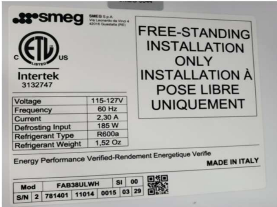
"Made in Italy", the model, and serial numbers are printed on a white label inside of the refrigerator's top door
